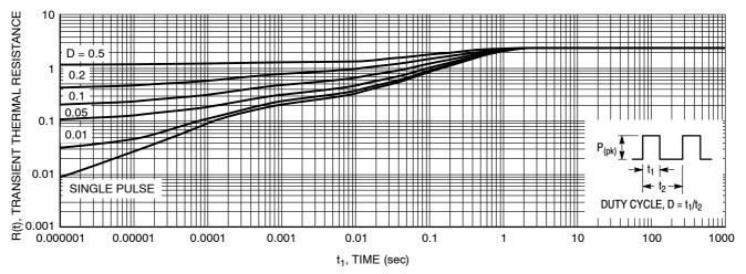
Figure 10. Thermal Response Junction-to-Case for MBRF20H100CT
