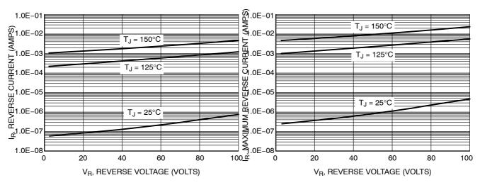
Figure 3. Typical Reverse Current
