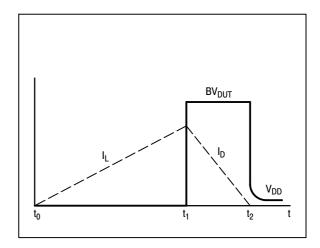
Figure 12. Current-Voltage Waveforms
