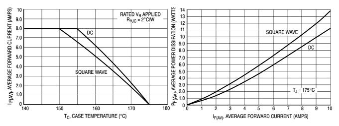
Figure 3. Current Derating, Case, Per Leg
