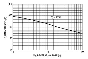
Figure 6. Typical Capacitance, Per Leg
