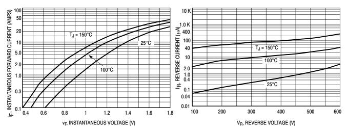
Figure 1. Typical Forward Voltage, Per Leg
