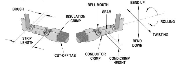
The above terminal drawing is a generic terminal representation. It is not an image of any terminal listed in the scope.
