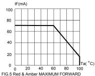
DC CURRENT VS AMBIENT TEMPERATURE (Tjmax=120°C)
