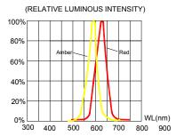
FIG.4 RELATIVE LUMINOUS INTENSITY VS. WAVELENGTH.
