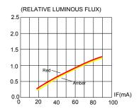
FIG.2 RELATIVE LUMINOUS FLUX VS. FORWARD CURRENT
