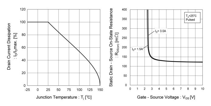
Fig.11 Drain Current Derating Curve
