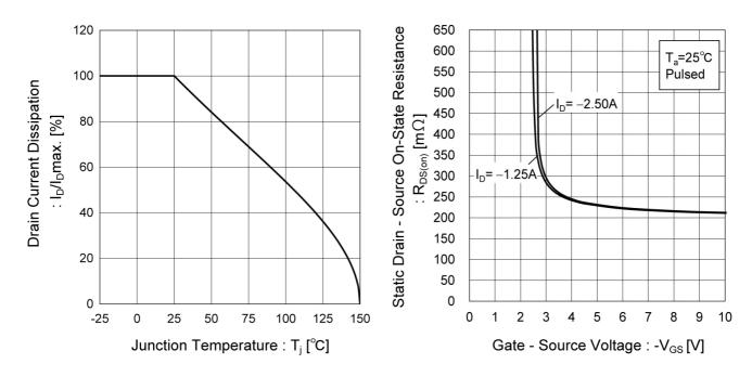
Fig.11 Drain Current Derating Curve
