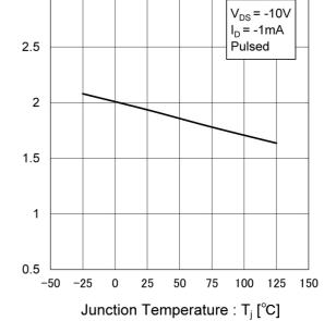
Gate Threshold Voltage : -V $_{GS(th)}$  [V]
