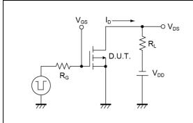
Fig.4-1 Gate Charge Measurement Circuit
