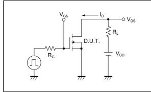
Fig.2-1 Gate Charge Measurement Circuit
