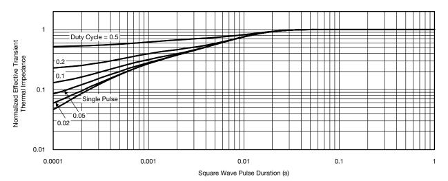
Normalized Thermal Transient Impedance, Junction-to-Case
