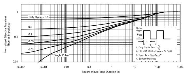
Normalized Thermal Transient Impedance, Junction-to-Ambient
