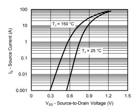
Source Drain Diode Forward Voltage
