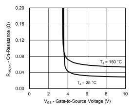
**On-Resistance vs. Gate-to Source Voltage**
