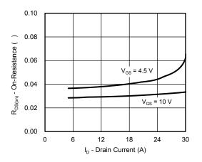
**On-Resistance vs. Drain Current**
