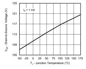
Drain Source Breakdown vs. Junction Temperature
