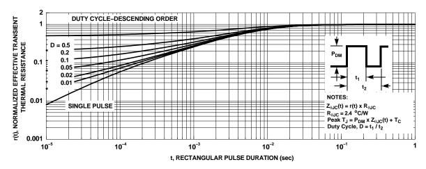
Figure 13. Junction-to-Case Transient Thermal Response Curve
