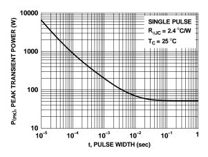
Figure 12. Single Pulse Maximum Power Dissipation
