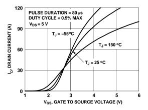
Figure 5. Transfer Characteristics
