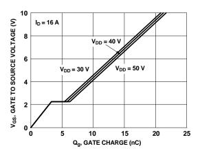
Figure 7. Gate Charge Characteristics
