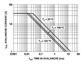
Figure 9. Unclamped Inductive Switching Capability
