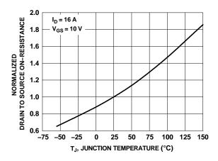
Figure 3. Normalized On-Resistance vs. Junction Temperature
